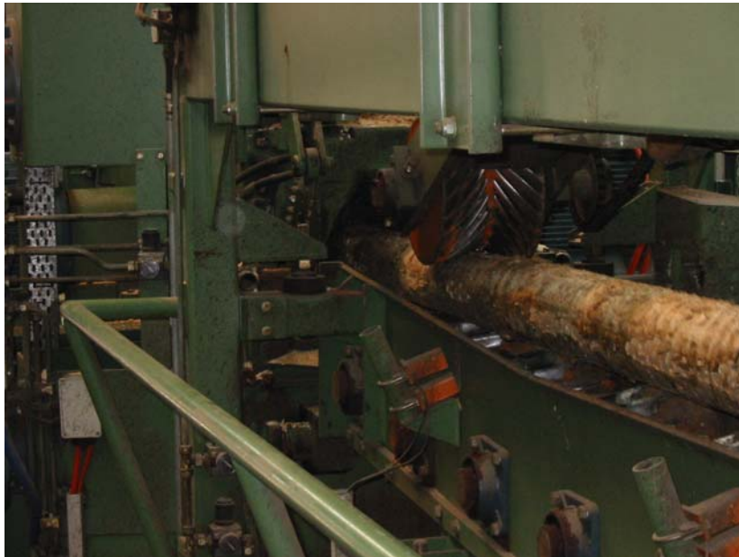
Figure 4-3: Log entering Hew Saw
